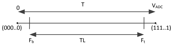
Fig. 2: Figure showing the total range, T (Codes 000...0 to 111...1) and the linear input range, TL ( F_t to F_b ) of ADC. T = TL if, F_t = 111..1 and F_b = 000..0 .
