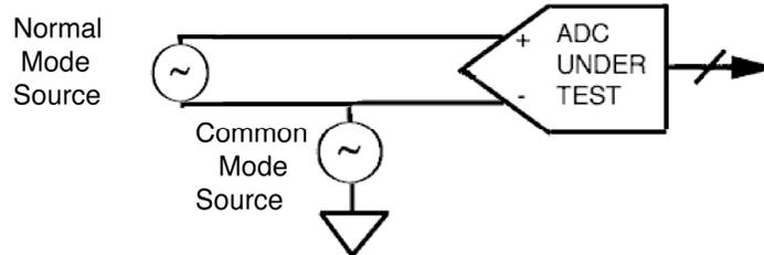
Figure 33—Block diagram of maximum operating common-mode signal
