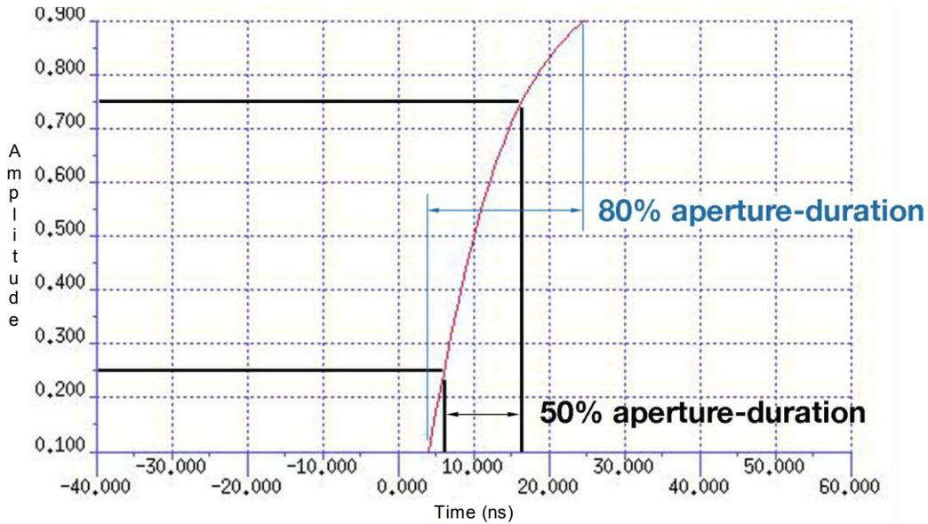
Figure 25—Aperture duration for  $p = 50\%$ , and  $p = 80\%$
