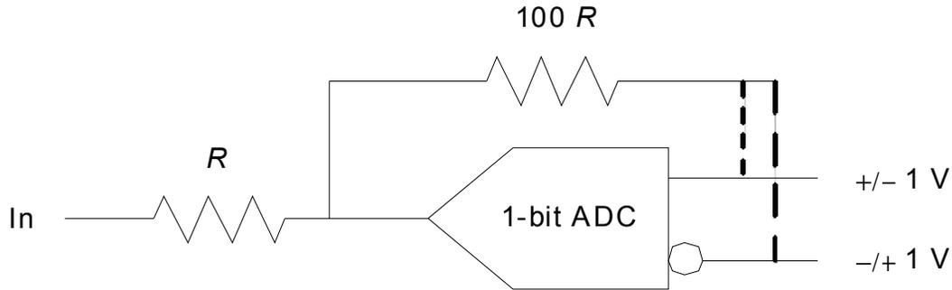
**Figure 13—Block diagram to demonstrate hysteresis and alternation**
