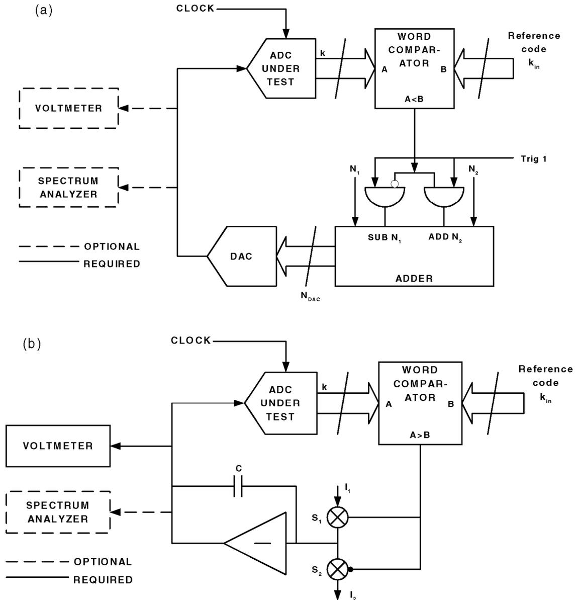
**Figure 9—(a) Block diagram of feedback loop (digital method);
