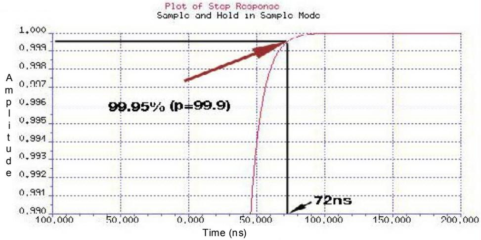
Figure 26—Evaluation of aperture-duration stop time for  $p = 99.9\%$
