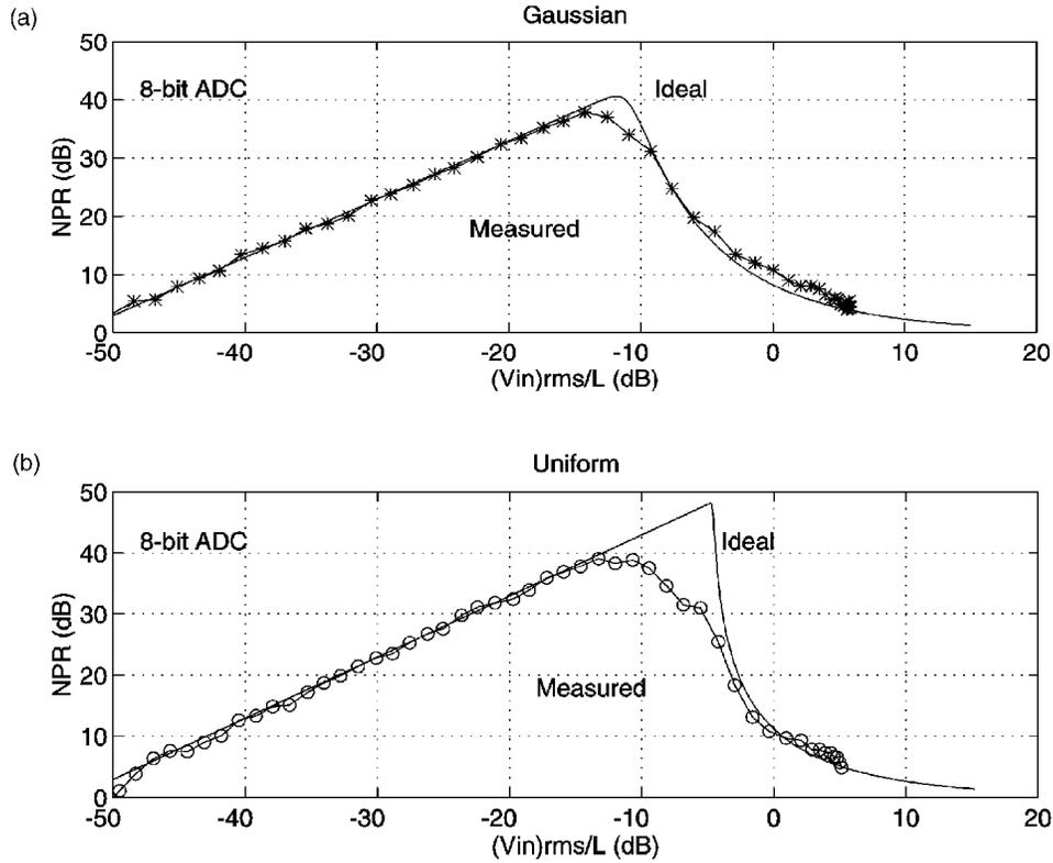
Figure 19—(a) Plot of ideal and measured NPR for a Gaussian noise input from Equation (63);
