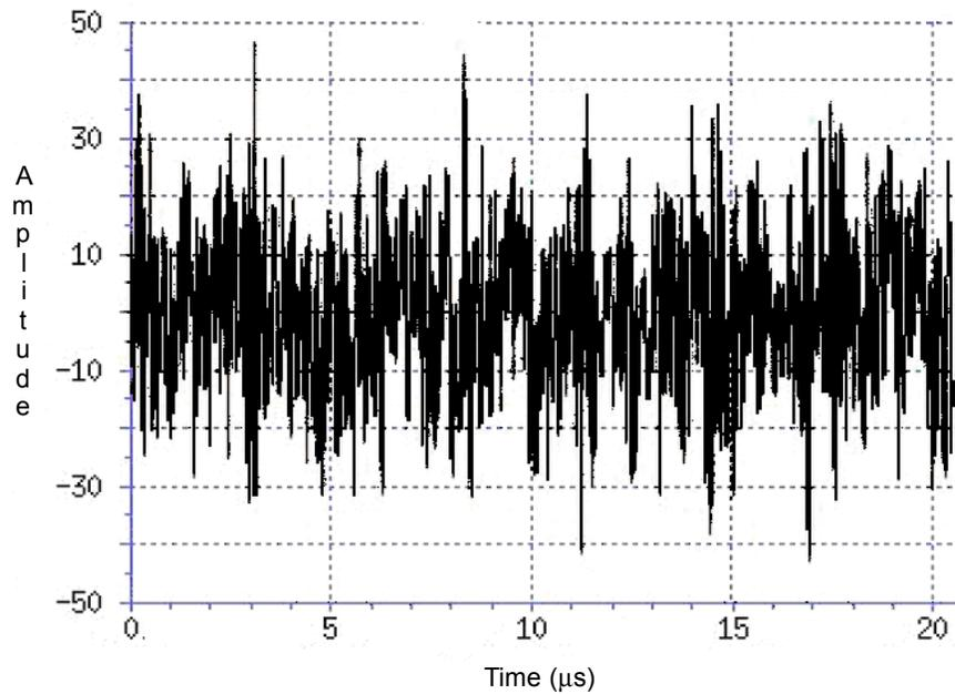
Figure 18—Time domain representation of NPR test signal
