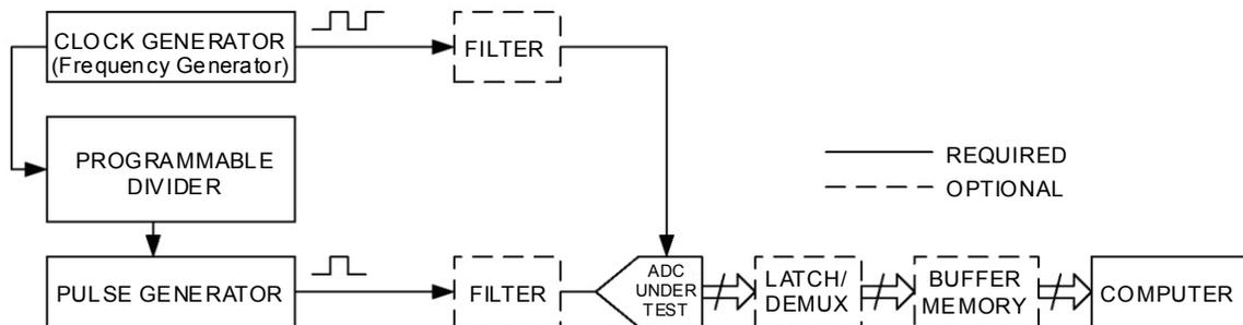
Figure 6—Setup for pulse and step signal testing
