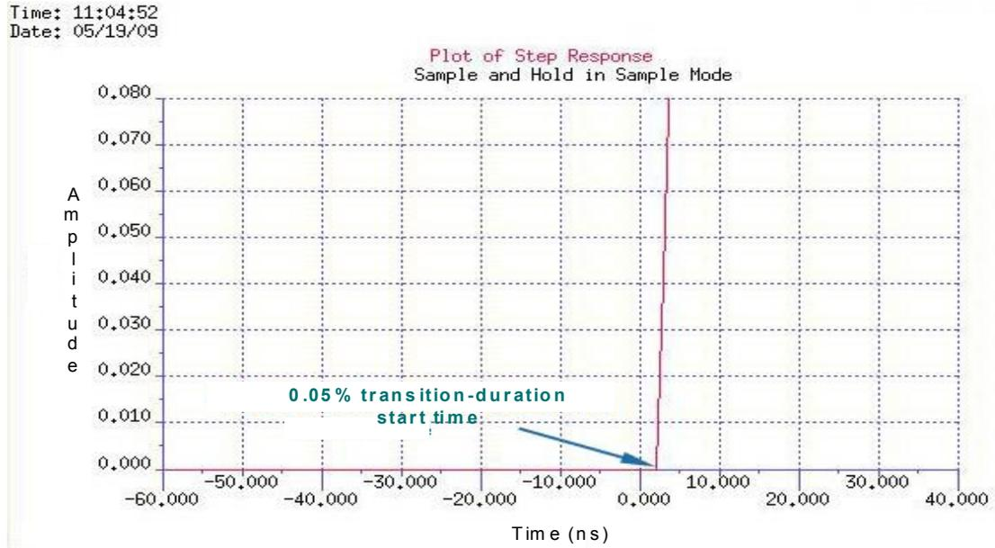
Figure 24—View of start of transition-duration for  $p = 99.9\%$
