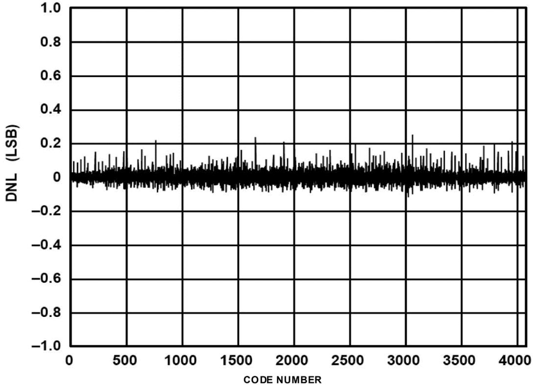
Figure 12—DNL from a terminal-based calibrated 12-bit device
